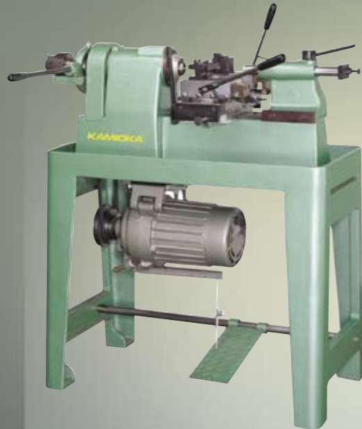
▲ Tool holders equipped at front & rear side
