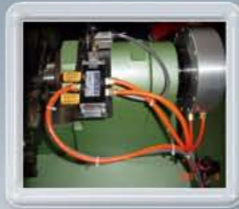
▲ Pneumatical auto. Clamping device
