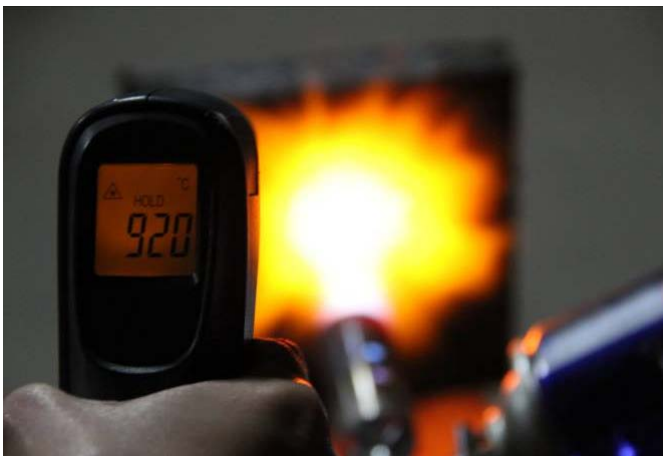
A 20 mm-thick straw panel made of FRG-M burning for 40 minutes, temperature measured 920 °C.
