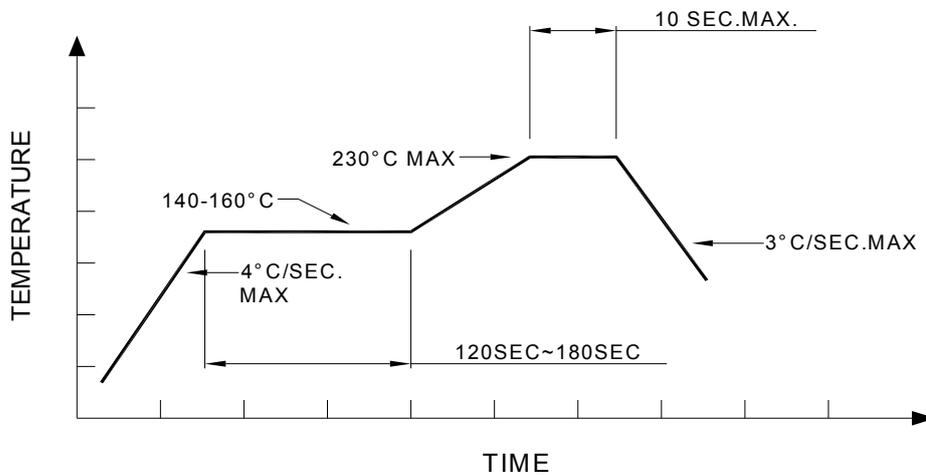
**Recommended Pb-free re-flow soldering profile:**
