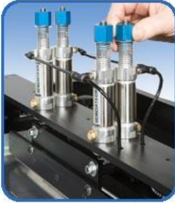
Squeegee blade pressure adjustment
