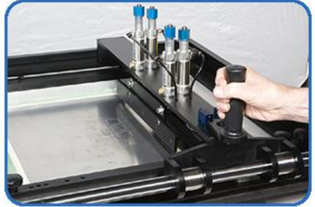
Dual squeegee side-to-side blade shuttle
